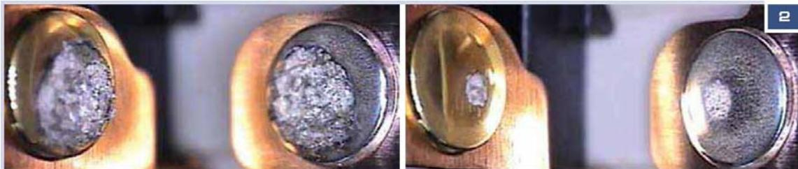
**Fig. 2.** (Left) Relay DE1a-L2-5V, which was used to switch a 440- $\mu$ F capacity and a 25-W discharge lamp on and off at random time points, welded shut after 1993 switching cycles. (Right) Same as left, but with phase-controlled switching used at current zero crossing; the zero crossing point was determined by adjusting several switch cycles in both directions. In the expectation of a long contact life, switching was terminated after 13,600 cycles.
