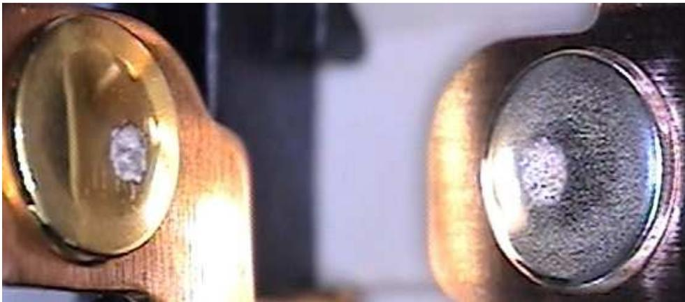
**Fig. 4b.** Same as Fig. 4a, but with phase-controlled switching used at current zero crossing; the zero crossing point was determined by adjusting several switch cycles in both directions. In the expectation of a long contact life, switching was terminated after 13,600 cycles.
