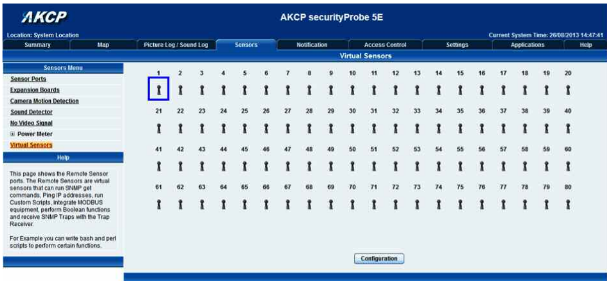
Figure: Here you see the 80 virtual sensors of the AKCP der securityProbe
